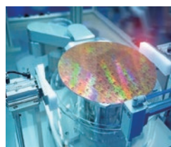
Example of cleaning process in semiconductor manufacturing
