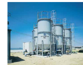
Upflow moving-bed filtration system
