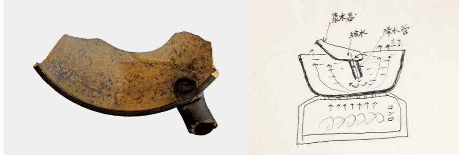
A sesame-toasting device used in boiler water circulation experiments along with a corresponding sketch
