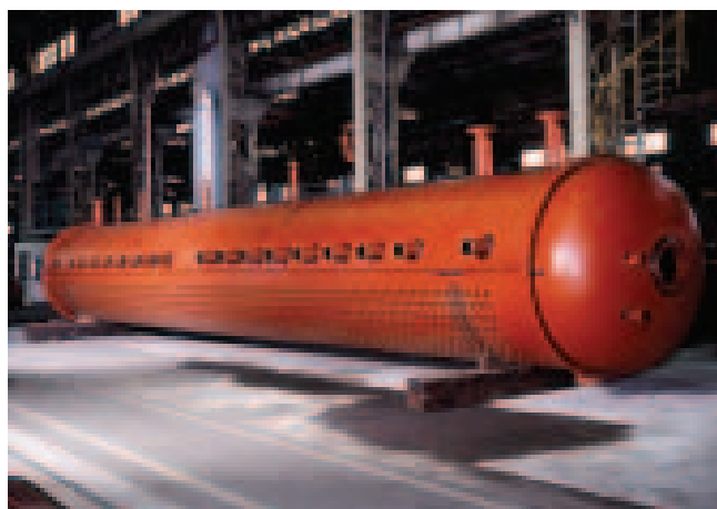
Drum of Water Tube Boiler
