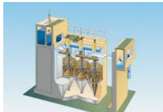
Intensive Sewage Treatment Filtration Facility
